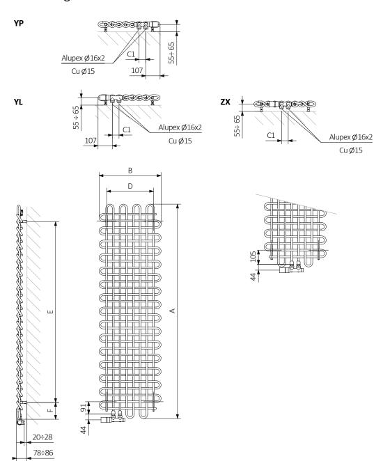
$A-Height \quad B-Width \quad C1-C5-Distance \ between \ pipe \ centres \quad D-Horizontal \ distance \ between \ mounting \ bracket \ centres \\ E-Vertical \ distance \ between \ mounting \ brackets \quad F-Distance \ between \ a \ mounting \ bracket \ and \ the \ bottom \ of \ the \ radiator$
