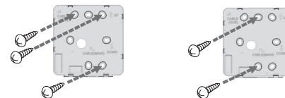
<4 socket reclamation box installation>
