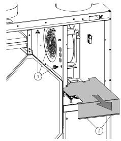
3. Insert reheater, lead cables trough holes on the side (pos. 1).
