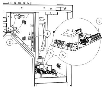
4. Place back covers of reheater and the main circuit board and secure them with screws.
