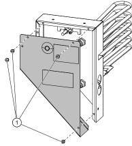
2. Remove knobs in the reheater compartment (pos. 1), they will be used to hold the reheater in place. Remove the main circuit board cover plate by removing 2 screws (pos. 2) in the lower front edge of the plate.
