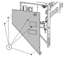
2. Remove 4 knobs in the reheater compartment (pos. 1), they will be used to hold the reheater in place. Remove the main circuit board cover plate by removing 2 screws (pos. 2) in the lower front edge of the plate.
