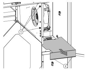
3. Insert reheater, lead cables trough holes on the side (pos. 1).
