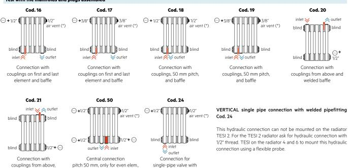
**CAUTION:** these configurations (Cod. 18 and Cod. 19) are not suitable for insertion of the integrated vale (for insertion of the integrated valve, see configurations Cod. 25 and Cod. 26).
