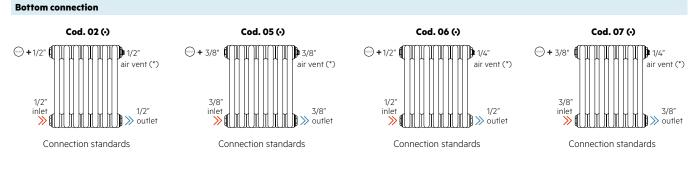
$\bullet$  For TESI radiators lower than 1000 mm or radiators with more than 15 sections.
