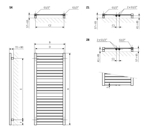
A – Height B – Width C1-C5 – Distance between pipe centres D – Horizontal distance between mounting bracket centres E – Vertical distance between mounting brackets F – Distance between a mounting bracket and the bottom of the radiator
